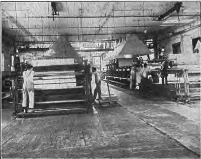
FIG. 138.—The cutter end of a Fourdrinier paper machine. (Courtesy of B. D. Rising Paper Co.)
